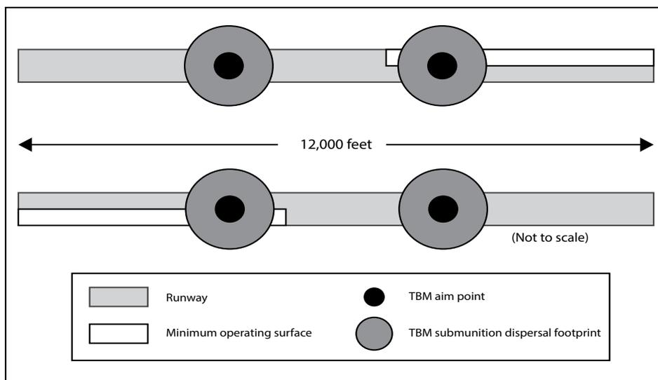
**Figure 3. Illustration of runway cut points**
